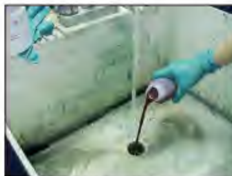
Figure 63: Dye Testing Plumbing (NEIWPCC, 2003)
